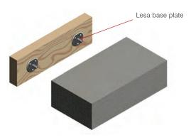
STEP 4: Strip the form. This is best accomplished by starting at one end and working along the form. Forms with base plates attached should be cleaned and stored for reuse.
