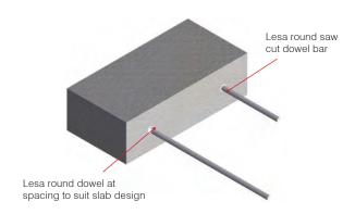
STEP 5: Insert the burr free end of the dowel bar into the Sleeve. Second concrete pour can now proceed.
