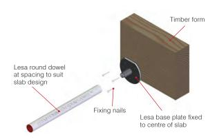
STEP 1: Mark the form for slab centre and sleeve spacing. Using three suitable nails or screws fix the sleeve base plate to the form.
