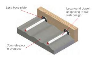
STEP 3: Place and finish the concrete. Edge of slab must be vibrated to consolidate concrete around the sleeve. (Care must be taken to ensure the sleeve is not dislodged).
