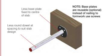
STEP 2: Set the form to line and level as normal. Slide the sleeve onto the base ensuring that it is flush with the base plate. Dowel support may be required to ensure the sleeve is not dislodged during placement.
