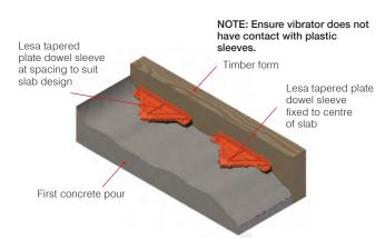
STEP 2: Set the form to line and level as normal and finish concrete. Edge of slab must be vibrated to consolidate concrete around the tapered dowel sleeve.
