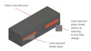
STEP 3: Strip the form. Forms should be cleaned and stored for reuse. Insert the tapered plate dowel when required prior to concrete pour.
