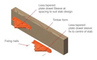
STEP 1: Mark the form for slab centre and tapered dowel sleeve spacing. Nail the sleeves to the form using the nails supplied in the sleeves.
