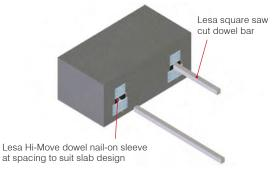
STEP 5: Insert the burr free end of the dowel bar into the nail-on sleeve. Second concrete pour can now proceed.
